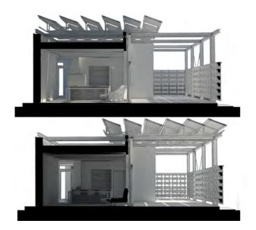
passive solar design for a mixed climate. Our house faces directly south and is long and thin on the east west axis. In the winter southern glazing allows low winter sun to access interior mass while in the summer that same mass takes heat out of the air to help stabilize the interior environment when diurnal temperature swings allow for some kind of night flush.
