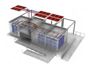
related volume of our thermal mass in the passive solar context, we have been able to implement a hybrid passive/active hydronic radiant heating and cooling system that, unlike conventional hydronics, uses only pump energy to accomplish temperature changes.
