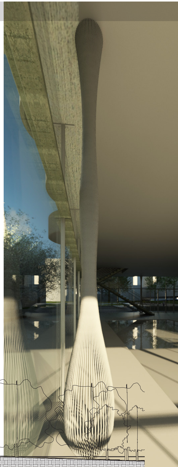
CHARLOTTE CONDO PROJECT. Academic exercise in advanced BIM design. Model built using custom parametrics families including adaptive component, curtain panel pattern based, and other family types.
