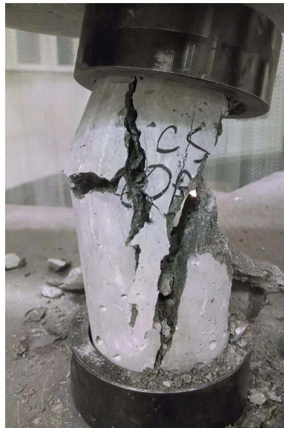
TESTING. Compressive strength: axial load application (left); thermal conductivity: modified transient plane technique (right); specific heat: differential scanning calorimetry (below)
