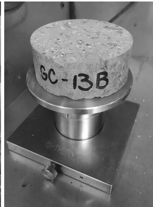
TESTING. Compressive strength: axial load application (left); thermal conductivity: modified transient plane technique (right); specific heat: differential scanning calorimetry (below)
