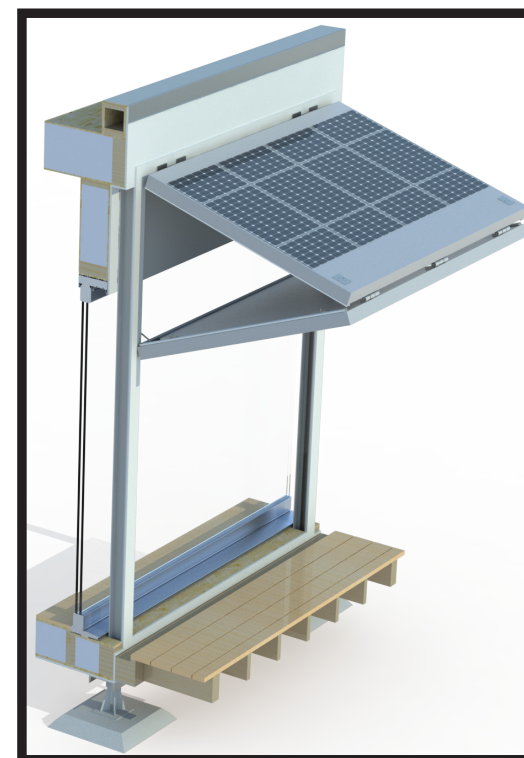
Panel gaskets compress against steel columns to create water-tight seal. Integrated solar panels are part of a direct DC water-heating system that supplies hot water even during a grid power outage.
