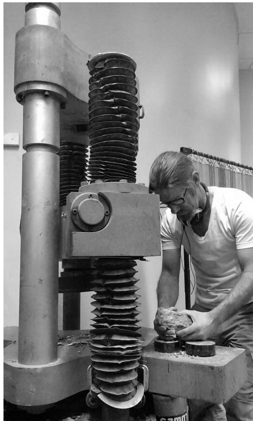
TESTING. Compressive strength: axial load application (left); thermal conductivity: modified transient plane technique (right); specific heat: differential scanning calorimetry (below)
