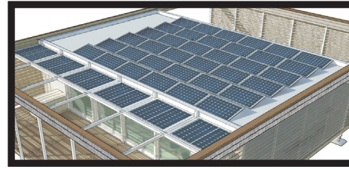
Resilient PV system engineered to produce energy for the neighborhood in the event of power outages.
