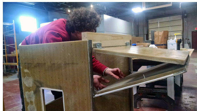
A model of the first envelope design direction: composite SIPs. This solution eventually fell prey to code restrictions.
