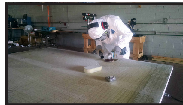
Custom glassfiber laminates were engineered and manufactured for specific flood loading...
