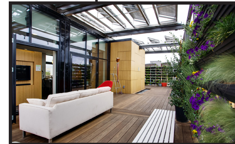
...and living room moves outside. Outdoor rooms double square footage of living space with living walls and movable PV array shading device.
