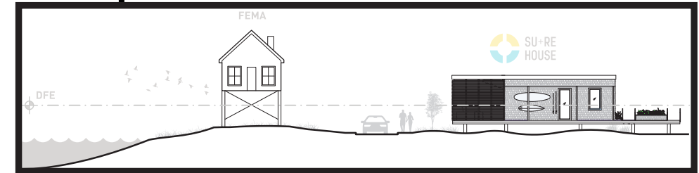
...part of a resilient design strategy to allow the building to be constructed in a backbay floodzone as an answer to FEMA's changes in regulations after Superstorm Sandy.
