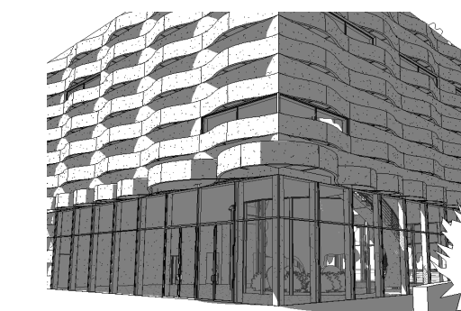
On August 30th at 1:00 the stationary horizontal overhangs fully shade the storefront glazing. This is the hottest time of the year in Charlotte 1/2 months after solstice with the sun well below it's apex.
